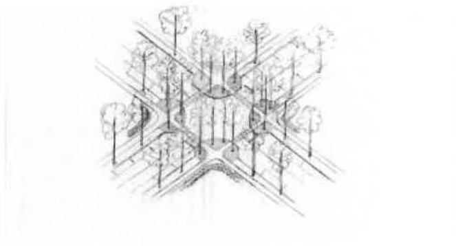
Nubs: Street corners may be extended to slow traffic by forcing a 90° turn. This will shorten the crossing distance for pedestrians.
