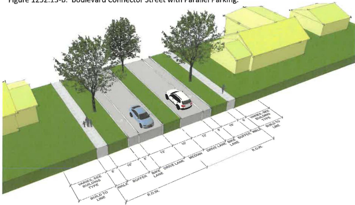
Figure 1252.13-B. Boulevard Connector Street with Parallel Parking.
